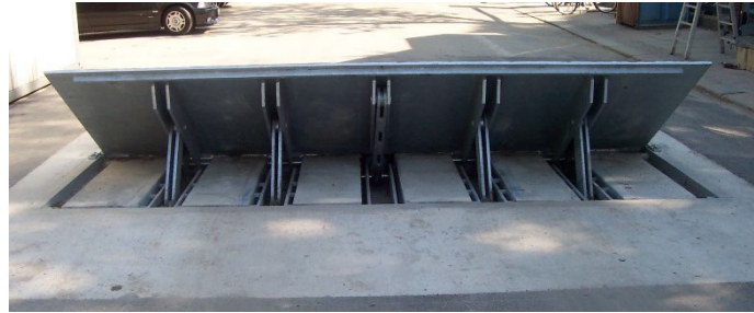
We are testing for your safety. A lorry (15.000 lbs) drives with a speed of 50 mph against the barrier.
