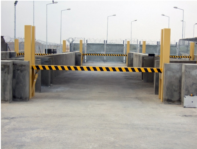
Secure access control by the combination of several drop arm barriers.
