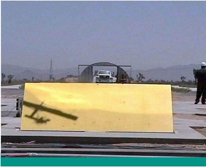
We are testing for your safety. A lorry (15.000 lbs) drives with a speed of 50 mph against the barrier.
