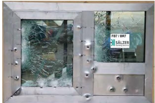
Result of the test: Classification in class **FB7-NS**. The complete window was tested with a gun calibre 7,62 x 51 steel hard core. The bullets have entered the outer profile and the glazing, **but did not come out of the profile on the room side! No splinters = NS**. In particular the weak points were tested: e.g. glass fittings.
