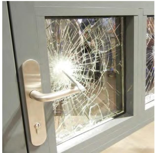
The P6B glazing can be pushed through within a few seconds. Therefore our glazed forced entry resistant doors which are equipped with anti-panic locks<sup>1)</sup> have glazing with integrated polycarbonate layer. The complete element is tested according to DIN EN 1627-1630.
