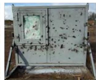
Steel partition and window after the successful test.
