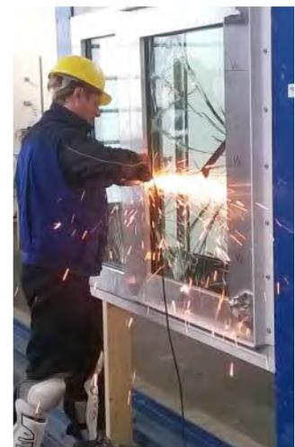
Aluminium window series S2es was tested with an angle grinder in the resistant class RC5.
