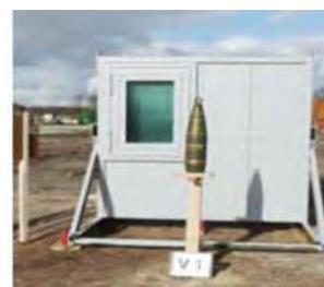
Test element with artillery shell, 43kg, was detonated in 1.5m.
