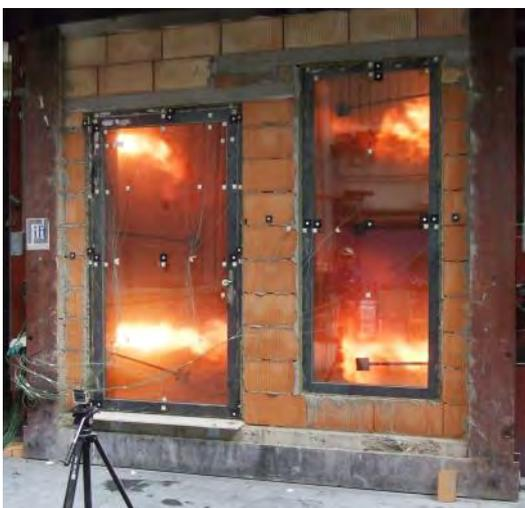
Multi functional door **SECUFIRE®** in the furnace, test EI45. Door is at the same forced entry resistant RC4 with anti-panic hardware, bullet resistant FB4-NS and tested in the explosive test with 500kg.
