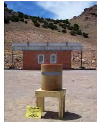
Open range according to UFC 4-010-02 (US Department of Defence) with 100kg TNT. Installation in masonry, this was similar to the later installation of the window on the construction site.
