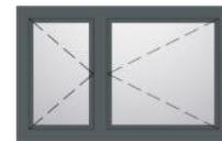
Inward opening turn window sash (right) to open for cleaning. Inward opening turn window sash (left), option perforated sheet outside.
