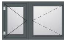
Inward opening turn window sash (right) to open for cleaning. Outward opening window sash (left), option: perforated sheet inside.
