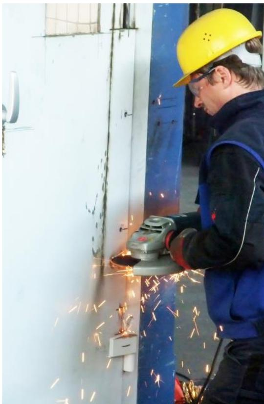
The examiner tries to destroy the inside bolts which lock into the frame with an angle grinder (discs Ø 230 mm).
