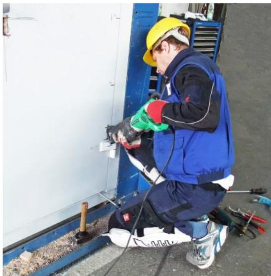
The examiner tried to saw off the hinges of the door with a sabre saw; without success as the certificate confirms.
